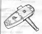
Place inner handle & mechanism on inside of door. Connect to outer handle with two metal thread screws.
