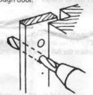
Place outer handle on door adjusting handle direction if necessary.
